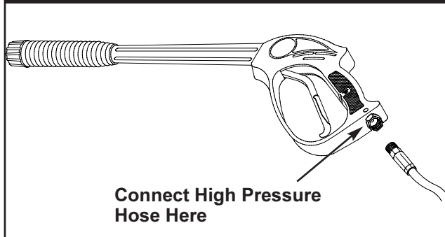
Figure 4 – Connect high pressure hose to spray gun.
